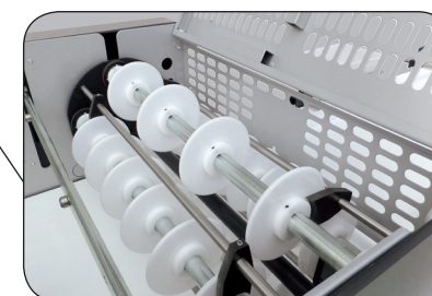
Longitudinal cutting disks and transversal cut guillotine.
